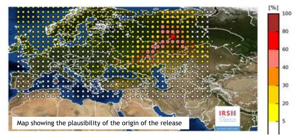
Map identifying, on the basis of the model-measurement comparison, the most plausible release zone. For a simulated release at each point of the mesh, the comparison consists in estimating the percentage of modelled data which are within a factor of 2 compared to actual measurements. The area with the highest percentage is identified as the most plausible release zone.
